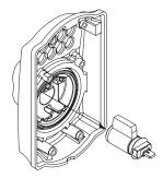
Remove Retainer, Block and Disc from Cylinder
